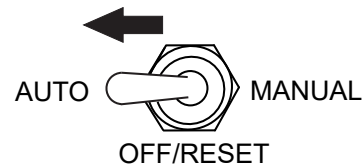
Figure 57. Auto Start/Stop Switch (Auto Position)
